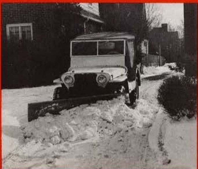
OPENING ROADS is another of the many jobs all in the stride of the mighty "Jeep." It is used successfully to plow sidewalks, driveways, city and town roads, and clean areas for service stations, manufacturing concerns. Four-wheel drive gives traction on icy roads.
