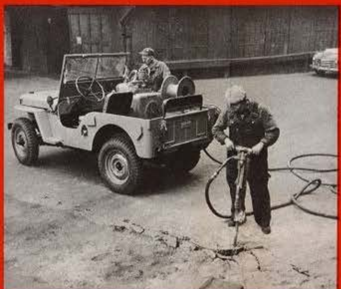
PORTABLE AIR COMPRESSOR supplies up to 60 cubic feet of free air per minute at 100 lbs. per square inch pressure, to power pavement breakers, rock drills, diggers, vibrators, riveting hammers, 6-gun paint sprayers, sand blasters, chain saws.
