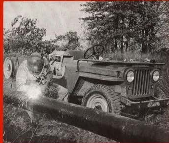
WHEN THERE'S WORK to be done, count on the "Jeep" being able to get there and do the job well! Here the mighty "workhorse of the world" is equipped with a 200 amp. welder mounted in the bed and operated from the center power take-off by V-belt drive.
