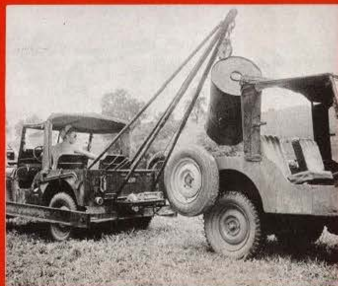
LIFTING a 600 lb. barrel of tar onto the bed of another "Jeep" is no trouble for this mighty workhorse of industry—the versatile Universal "Jeep." Equipped with a winch and crane, it also has a heavy-duty bulldozer mounted on the front end for added usefulness.
