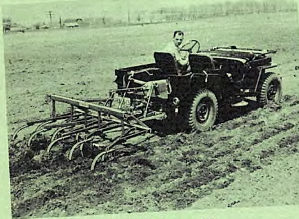
Newgren field cultivator with Monroe Lift stabilizer bars in certain soil conditions.
