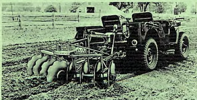
Views of the Newgren lift-type Bush and Bog Harrow in action, reworking hard, packed ground, and summer fallowing.
